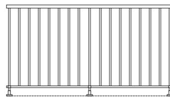
**Barandilla de barrotes total** | Guarda-corpo de grade integral | Barraudage sous main courante | Total railing with balusters
