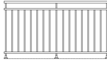
**Barandilla de barrotes con borde superior libre** | Guarda-corpo de grade com borda superior livre | Barraudage sous lisse intermédiaire | Railing with balusters and separated upper handrail
