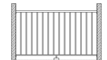
**Barandilla de barrotes total entre muros** | Guarda-corpo de grade integral entre paredes | Barraudage sous main courante entre murs | Total railing with balusters between walls
